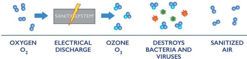
The Sanity System ozone generators are provided with the "Safe System", This system allows the conversion of residual ozone back to oxygen in a very short time frame making it safe for you to go back into the place of sanitization.
